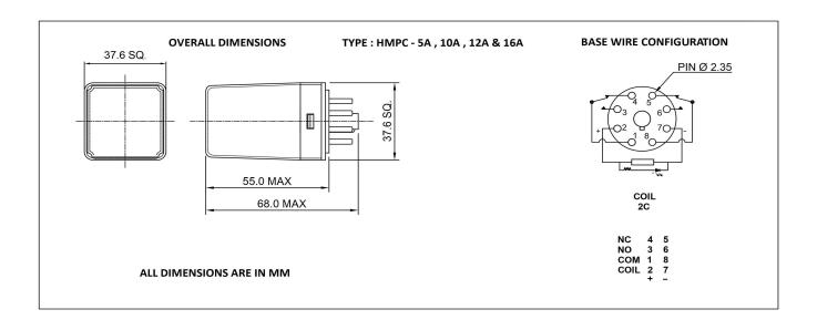
NOTE:-1) In case no tolerance shown in outline dimensions: Outline dimension 1mm, tolerance should be ±0.2mm
