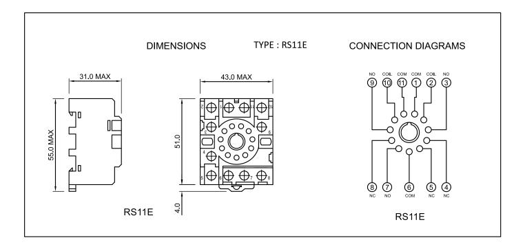
NOTE:-1) In case no tolerance shown in outline dimensions: Outline dimension 1mm, tolerance should be ±0.2mm Outline dimension 1mm and 5mm, tolerance should be ±0.3mm Outline dimension 5mm tolerance should be±0.4mm 2) The tolerance without indicating for PCB layout is always ±0.2mm
