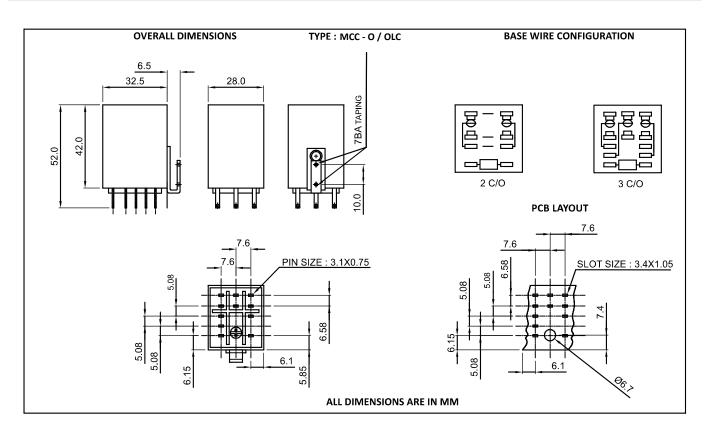
NOTE :- 1) In case no tolerance shown in outline dimensions : Outline dimension 1mm, tolerance should be ±0.2mm Outline dimension 1mm and 5mm, tolerance should be ±0.3mm Outline dimension 5mm tolerance should be±0.4mm 2) The tolerance without indicating for PCB layout is always ±0.2mm
